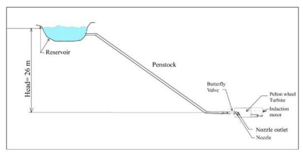
Figure 7: Schematic Representation of Micro Hydro Power Houses
