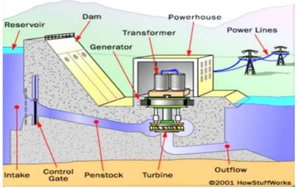
Figure 6: Schematic Representation of Major Hydro Power Houses
