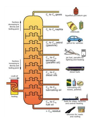
Figure 38: Fractional distillation of crude oil
